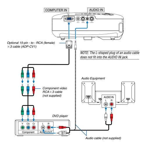
A component signal will be automatically displayed. If not, from the menu, select [Setup - Options]  $\rightarrow$  [Signal Select]  $\rightarrow$  [Computer], and then place a check mark in the "RGB/Component" radio button.
